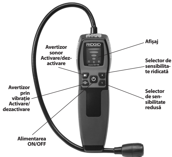
Figura 2 – Componentele micro CD-100
